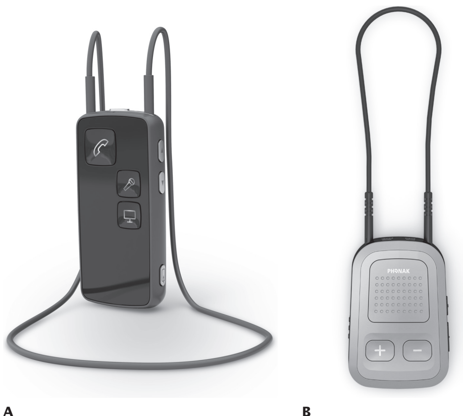
Figure 21-2. Streamers that communicate with hearing aids via nearfield magnetic induction. Sources: A. Photo courtesy of Oticon A/S. B. Image © Sonova AG. Reproduced here with permission. All rights reserved.
