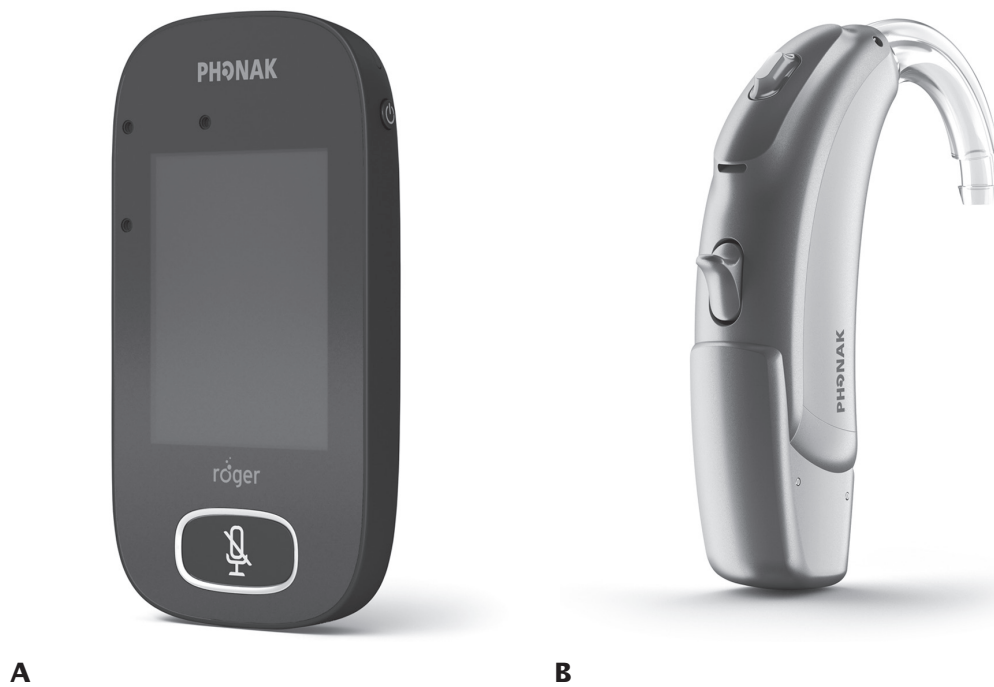
Figure 21–6. A DM transmitter (A) and integrated receiver attached to base of a hearing aid (B). Source: Images © Sonova AG. Reproduced here with permission. All rights reserved.
