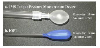
**Fig. 2.** Probes for tongue pressure measurement. a. JMS Tongue Pressure Measurement Device. b. Iowa Oral Performance Instrument.
