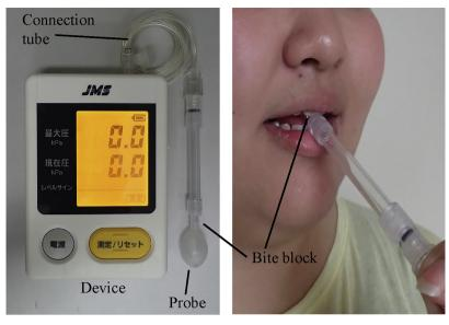
Fig. 1. JMS Tongue Pressure Measurement Device.
