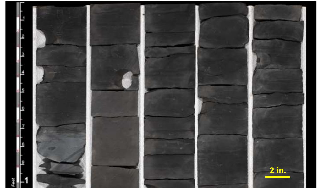
Organic-rich Wolfcamp D (Canyon – Cisco) black shales in core from the center of Midland Basin
