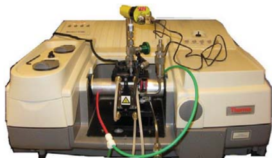
Figure 22: High-pressure high-temperature cell installed in the main compartment of a FT-IR spectrometer. Special adapters have been designed and machined in Al6061 to ensure a perfect N 2 purge of the system, so the water, hydrocarbon and CO 2 gas level out of the cell is kept constant.
