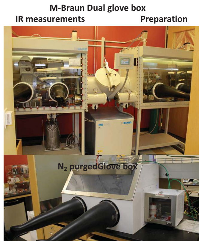
Figure 4: Top: M-Braun Dual glove box. The glove box on the right is use for sample preparation, the one on the left contains an FT-IR spectrometer for characterization. Bottom: Small N2 purge glove
