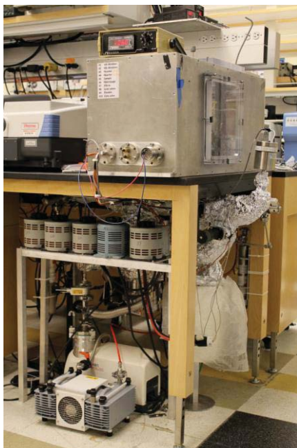
Figure 13: UHV chamber #5. The UHV reactor is enclosed into an Aluminum box continuously purged with N 2 gas. In that Al box are also located the parabolic and ellipsoidal mirror and the IR detector. Pumps, vacuum gauges and gas inlets are out of the box, below the table.
