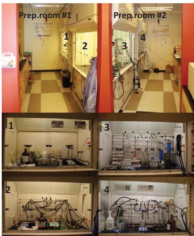
Figure 3: top: two Chemical preparation rooms each one equipped with two hoods and a DI water polisher. Bottom: view of the hoods.
