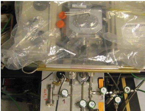
Figure 19: Custom-made all-aluminum reactors interfaced to IR spectrometers to study aggressive vapor phase processing of semiconductor and metal surfaces (e.g. \text{XeF}_2 etching). Sample holders have been built for transmission and reflection geometries, as well as gas phase spectroscopy.
