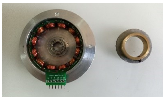
Fig. 7. The prototype stator and rotor of the 1-X resolver with CTNOW configuration.
