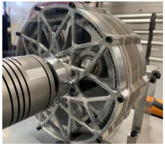
Fig. 10 The 50:1 tripartite rotor cycloidal magnetic gear POC prototype.
