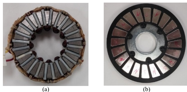
Fig. 5. (a) Tape Wound Stator and (b) Rotor of Repurposed Axial Flux PM Machine
