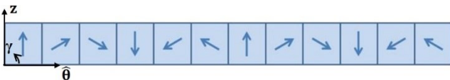
Fig. 2. Halbach Magnet Array (with N_P = 3 ) Focusing the Magnetic Field Below the Array (in the z- Direction)
