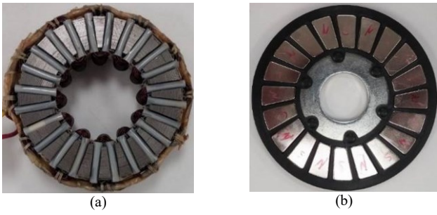
Fig. 5. (a) Tape Wound Stator and (b) Rotor of Axial Flux PM Machine
