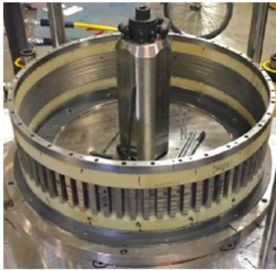
Fig. 8. (a) Simulated no load and maximum load (stall torque) leakage flux densities axially beyond the active stack in (b) the modulator assembly.
