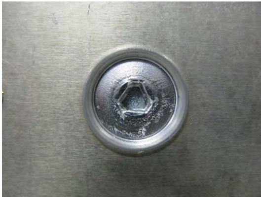
Fig. 17. The picture of the specimen after the tool suddenly stopped while welding for the concave triangular pin.
